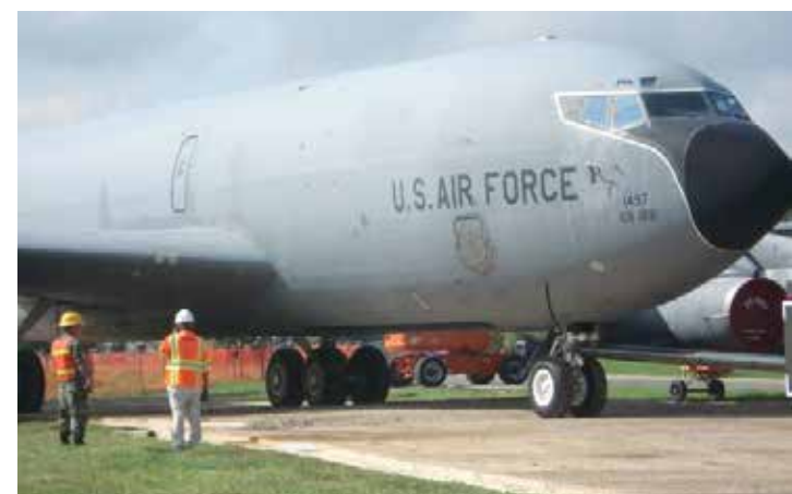
Mats help transport a 55-ton, KC-130 aircraft at a New Jersey airshow.
